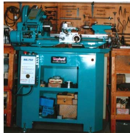
Inverter controller shown fitted to Myford ML7
